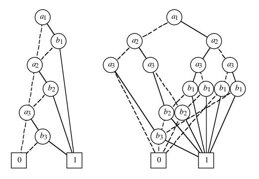
Figure 3: OBDD Representations of a Single Function for Two Different Variable Orderings.
