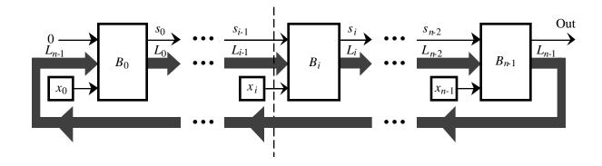
Figure 5: Linear Arrangement of Within-K Ring Circuit. As shown by the dashed line, the circuit has forward cross section  $2 + \lceil \log_2 K \rceil$  and reverse cross section  $\lceil \log_2 K \rceil$ .
